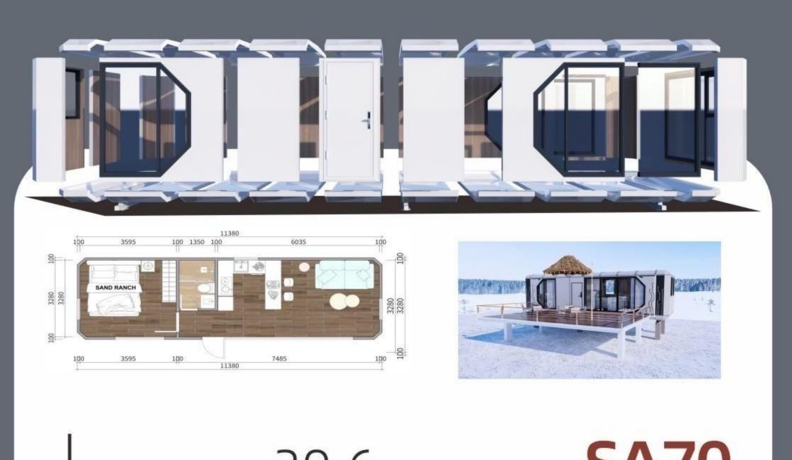
**SA70** Building area: 39.6 m² (Disassembled Type in 40HQ) Length: 11.3m
